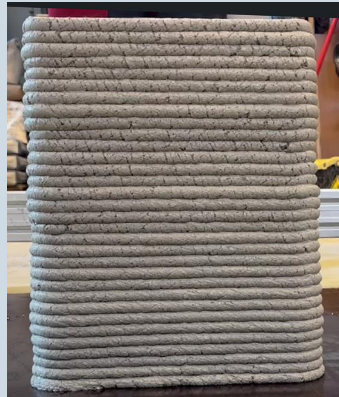
Fig. 1. A small-scale printed object using one of the developed GCP mixtures, indicating good buildability.
