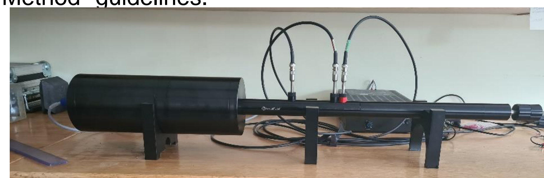
Fig. 2. Impedance tube used in measurements.
